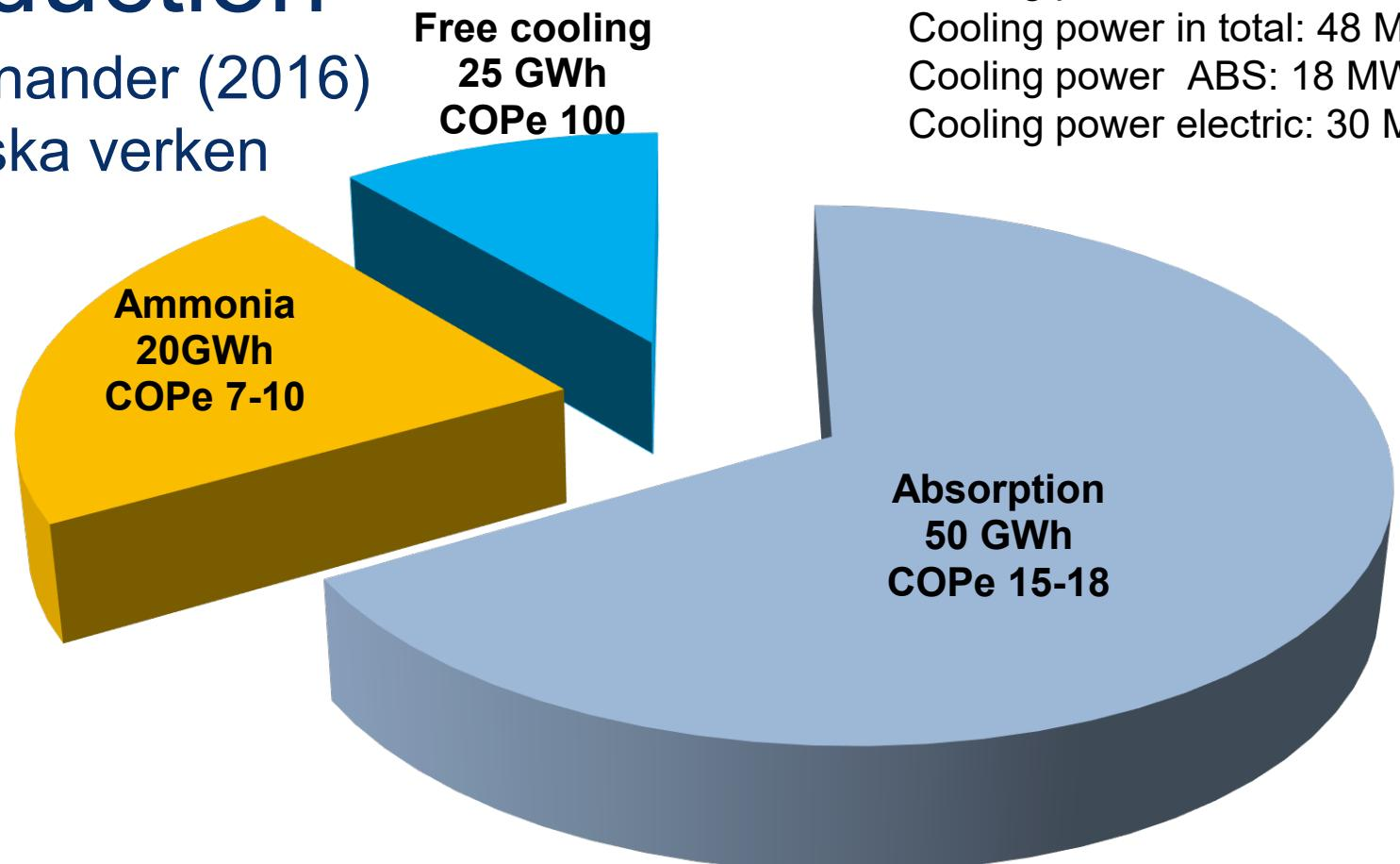
COPe= Coefficient of Performance, electricity to cooling
